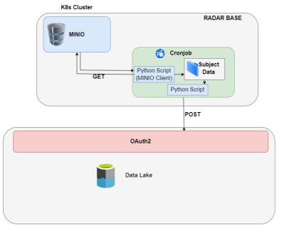
Figure 36 Architecture of data communication to the Data Lake mechanism.
