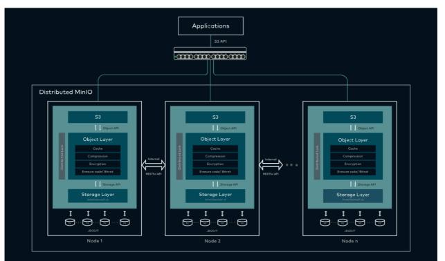
Figure 13 Distributed MinIO architecture on multiple service nodes [16].
