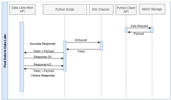
Figure 34 Posting Data to LETHE Data Lake sequence diagram, as developed by ExtraRed.
