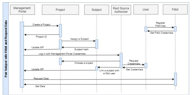
Figure 33 Pair Subject with Fitbit and Data request sequence diagram.
