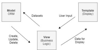
Figure 38 Model-Template-View design pattern, the backbone of the Django architecture.
