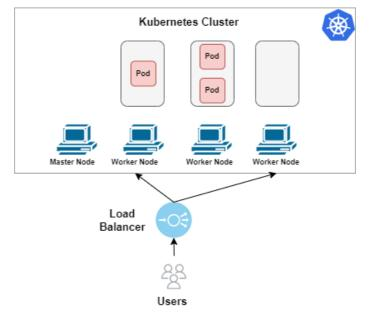
Figure 9 Load-Balancing service concept.
